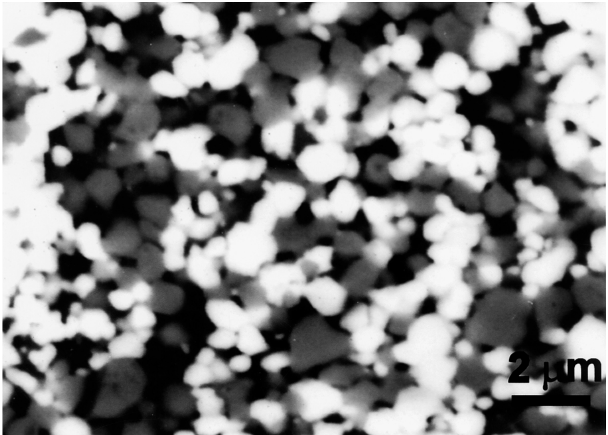
Figure 4 SEM microstructure of the mixture of the PZT and NiO powders, fired at 850°C. Dark grains are NiO, lighter grains are PZT.
